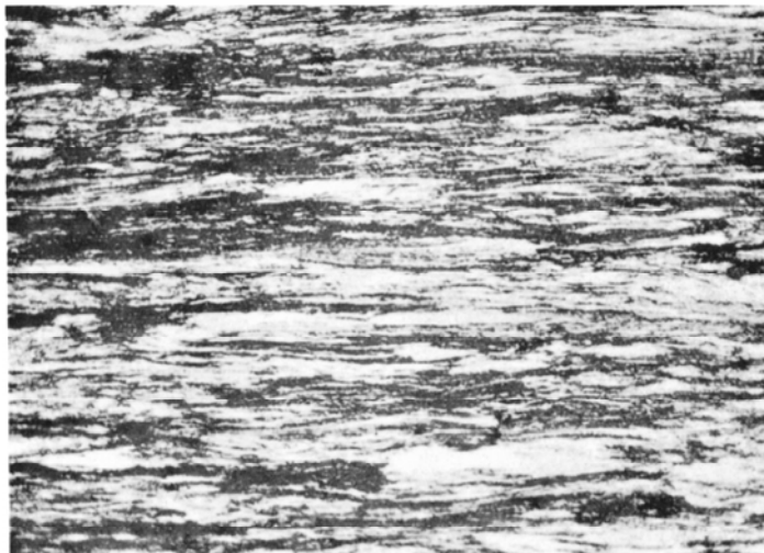
Fig.8 Metallographic structure of longitudinal section of patented hard drawn wire
