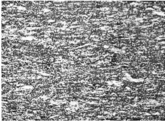
Fig.6 Metallographic structure of longitudinal section of hard drawn EN.49D range 2 wire
