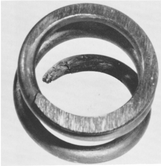
a. LOW FATIGUE LIFE (UNPEENED) SUPPLIER A
