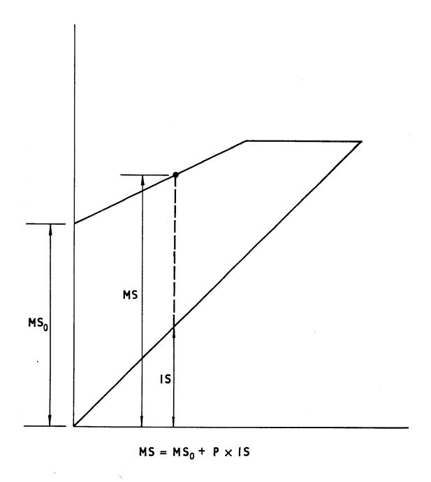
FIG. 1. EQUATION REPRESENTING GOODMAN DIAGRAM
