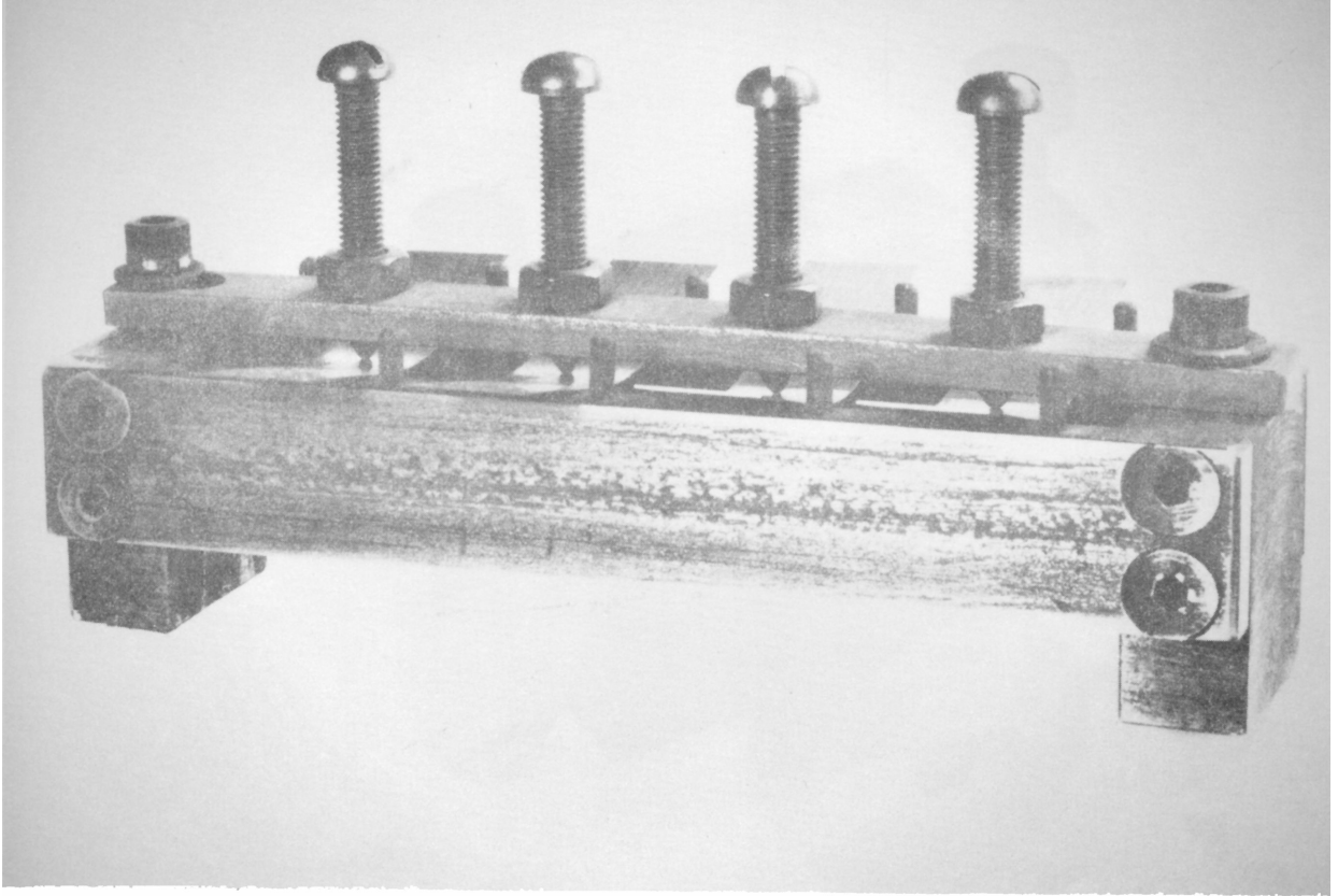
FIG. 12 Three Point Bending Jig for Stress Relaxation of Strip
