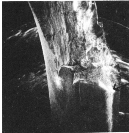
Fig 25 x 14 General appearance of fracture initiation due to corrosion, close to inside of spring coil
