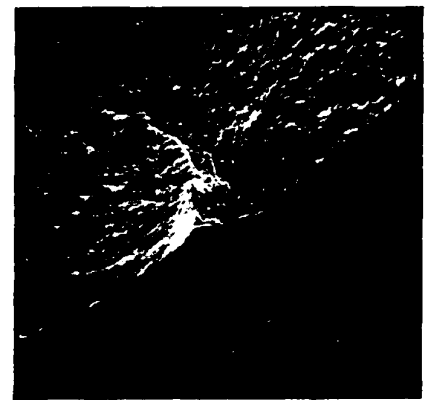
Fig 3. Shear crack parallel to wire axis - BS2056 302S26 gr 2 of 2.64 mm: range of torsional stress = 500 N/mm 2 ; number of cycles to failure = 1.2 × 10 6 ; magnification ×66
