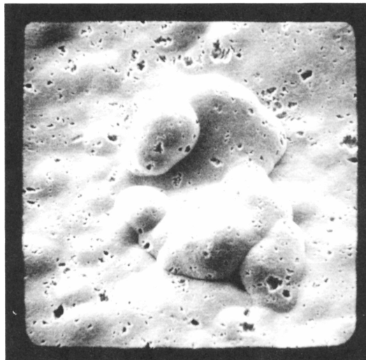
Fig 32 X 515 Detail of granular deposit at centre of spotted zone above (arrowed). Note also porosity of plate.
